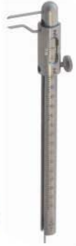
DE-1454 Gauge for measuring distances (0 - 90 mm),
